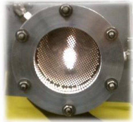
Fig. 1. PPA reactor chamber with hydrogen and methane plasma
