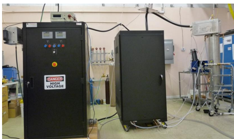
Fig. 1. High-pressure RF plasma system APT-100-2 for BNNT production and new materials synthesis.
