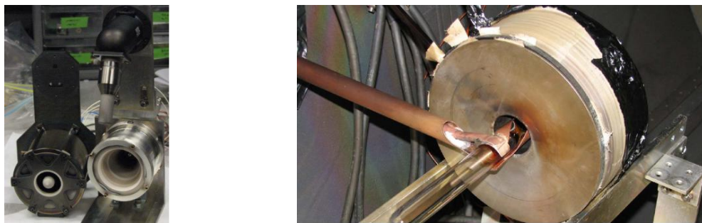
Fig. 1. BHT-200 and DCF Hall-effect ion thrusters (HETs) at the left (external cathode-neutralizer installed on the latter), and electrodeless Minihelicon plasma engine at the right
