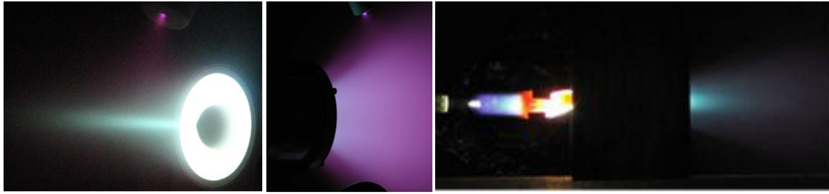
Fig. 2. Photos of HETs in-vacuum operation: (left) BHT-200 in high-voltage spike and DCF in the low-voltage diffuse mode (middle). Mini-helicon operation on Xe is shown in the right photo
